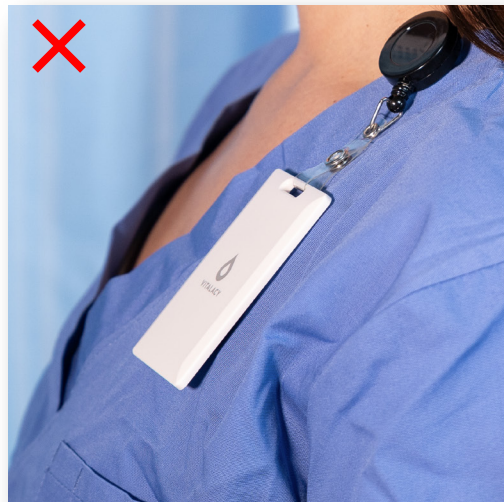
In this position, the SmartBadge has little space between the device and your chest, making it more difficult for the signal to be emitted.
