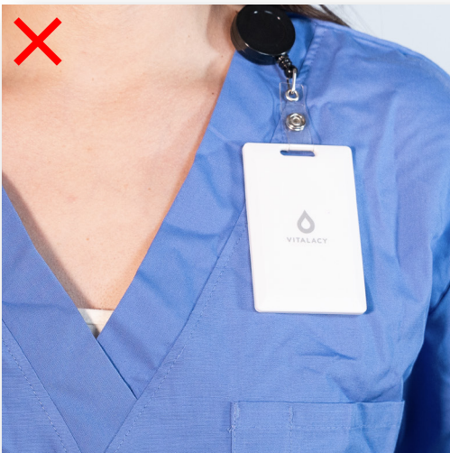
Wearing the device on your upper chest can also cause a weaker signal from the SmartBadge.
